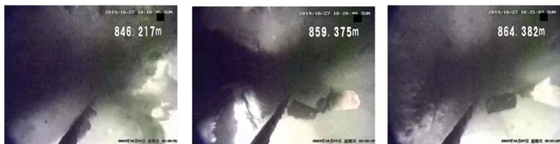
Fig. 4. Leak detection result of Well XX1 in Changqing Oilfield
